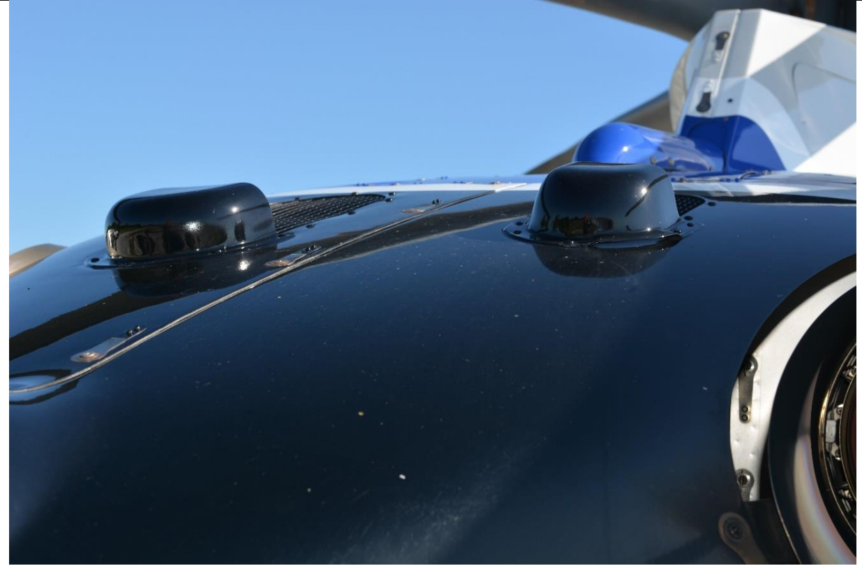
Photo IV-33 N461MT Rear Air Ducts Detail
