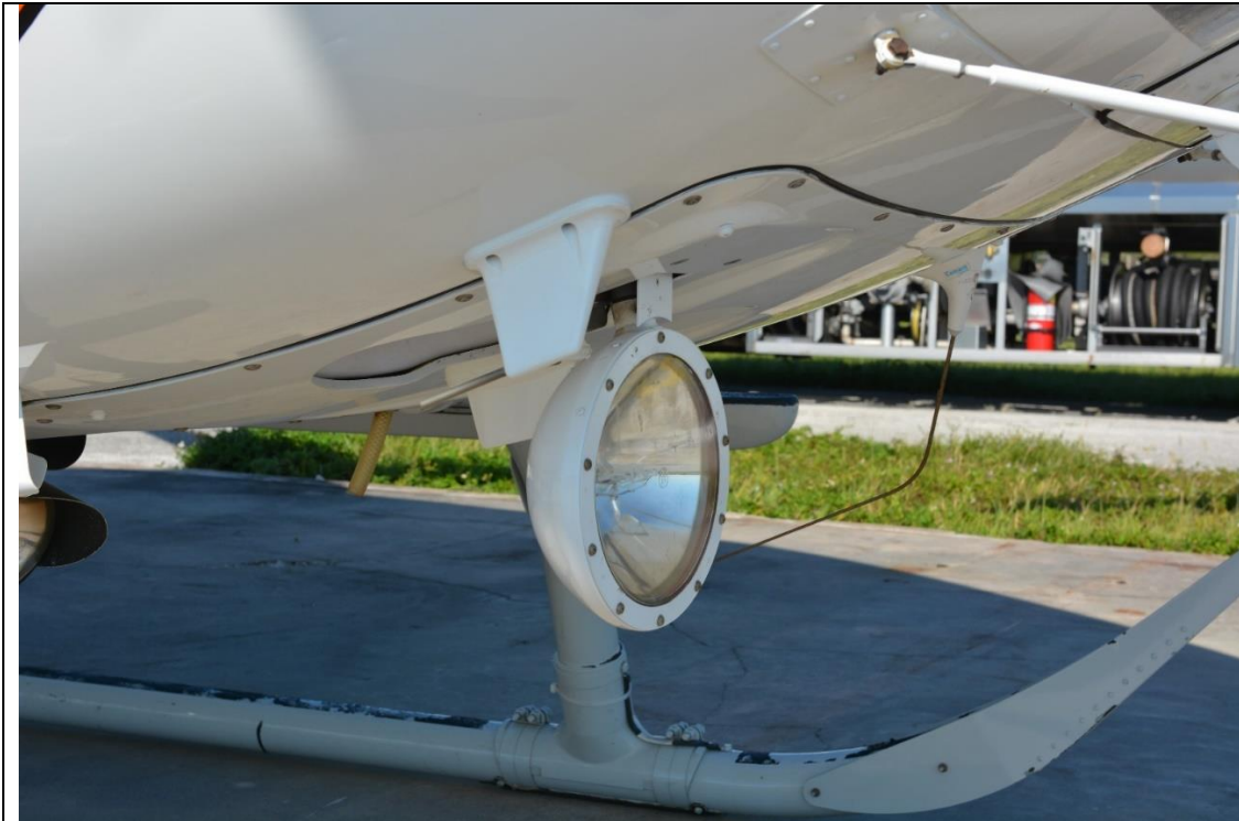
Photo IV-63 N461MT Operational Landing Light Detail
