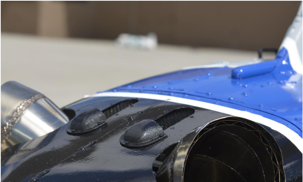
Photo IV-34 Replica Rear Air Ducts Detail
