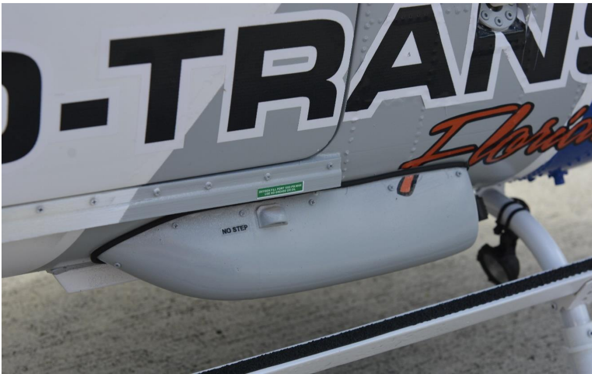
Photo IV-90 Replica Left Oxygen Tank Detail
