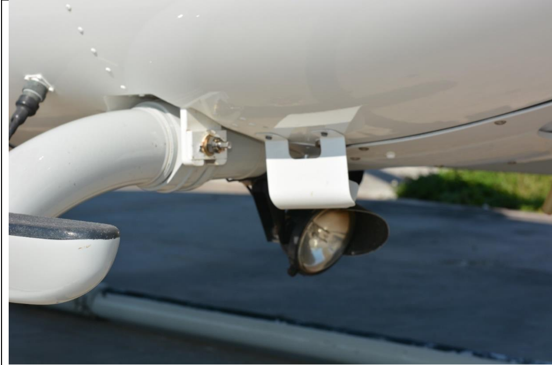
Photo IV-61 N461MT Right Lower Pitot Detail
