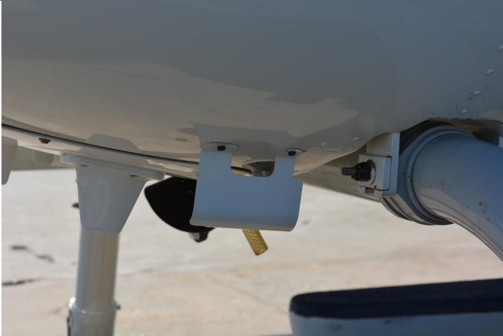
Photo IV-77 N461MT Left Lower Pitot Detail
