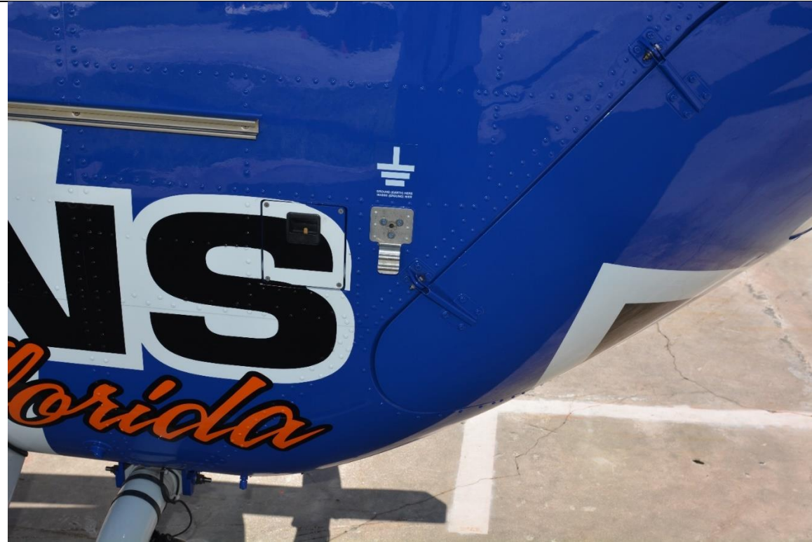
Photo IV-93 N461MT Ground Bar Detail
